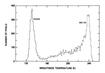
Figure A-2. Typical winter distribution of brightness temperatures in map elements (pixels) between 55°S and 65°S.
