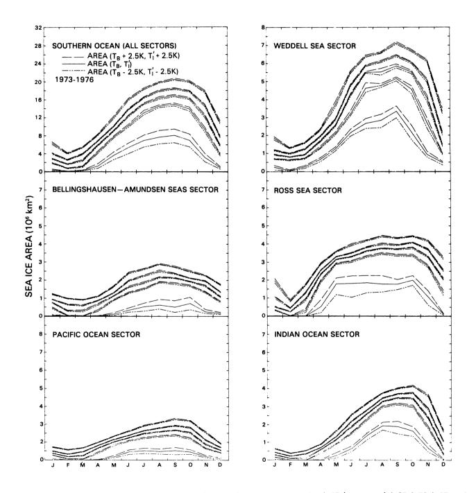
Figure 3-29. Sensitivity of the ocean area covered by sea ice with concentration  $\ge$ 15 (top curves),  $\ge$ 35,  $\ge$ 50,  $\ge$ 65, and  $\ge$ 85 percent (bottom curves) to a 2.5 K error in both the brightness temperature,  $T_B$ , and the estimated snow/ice interface temperature,  $T_I$  (see Figure 4-8).
