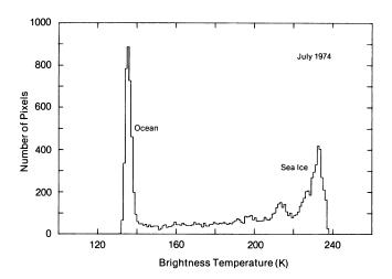
Figure 3-27. Distribution of brightness temperature derived from ESMR data in the Weddell Sea sector (60°W to 20°E) during July 1974.
