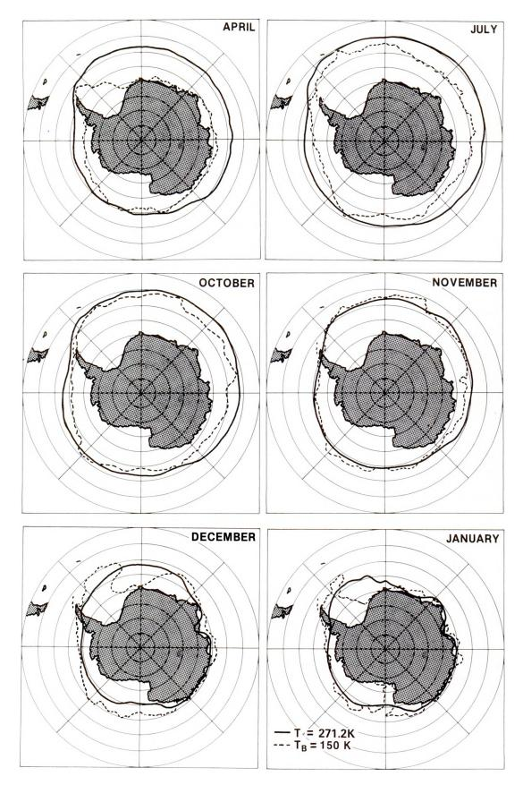
Figure 2-8. Comparison, for six selected months during the growth and decay seasons, of the 271.2 K freezing isotherm from climatological surface air temperatures with the position of the ice edge ( $T_B = 150 \text{ K}$ ) averaged for 1973-1976 (Chapter 3).
