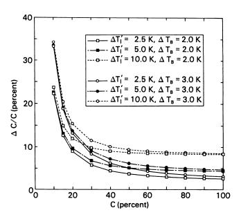
Figure 3-28. Uncertainty in ice concentration derived from ESMR data as a function of ice concentration, presented for several errors in brightness temperature ( $\Delta T_B = 2.0$  and 3.0 K) and for several errors in estimated snow/ice interface temperature ( $\Delta T_1' = 2.5$ , 5.0, and 10 K).
