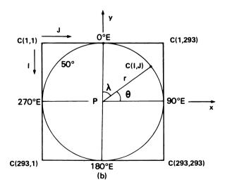
Figure A-4. Schematic diagram for polar stereographic mapping.
