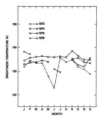
Figure A-3. Mean recorded brightness temperature of the ocean between 55°S and 65°S, plotted for each month, 1973 through 1976, before correction for calibration shifts.
