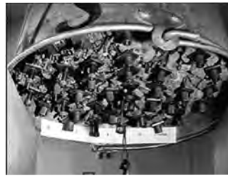
ABOVE: The bucket test – bucket filled with crushed rock and model rock bolts used to demonstrate the principle to tunnel workmen. Image courtesy SMEC collection.
