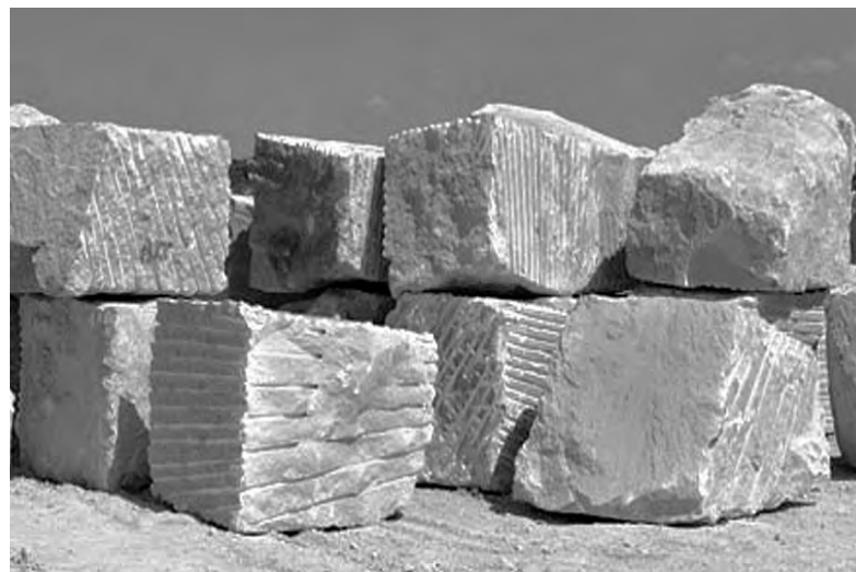
Portland Block Stone. Image courtesy Portland Stone Firms Limited, UK at http://www.stonefirms.com .
